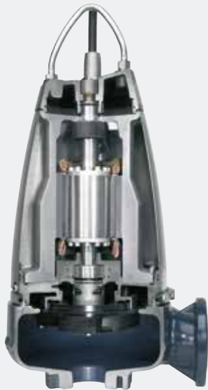
Fig. 5 Submersible sewage pump with SuperVortex impeller
