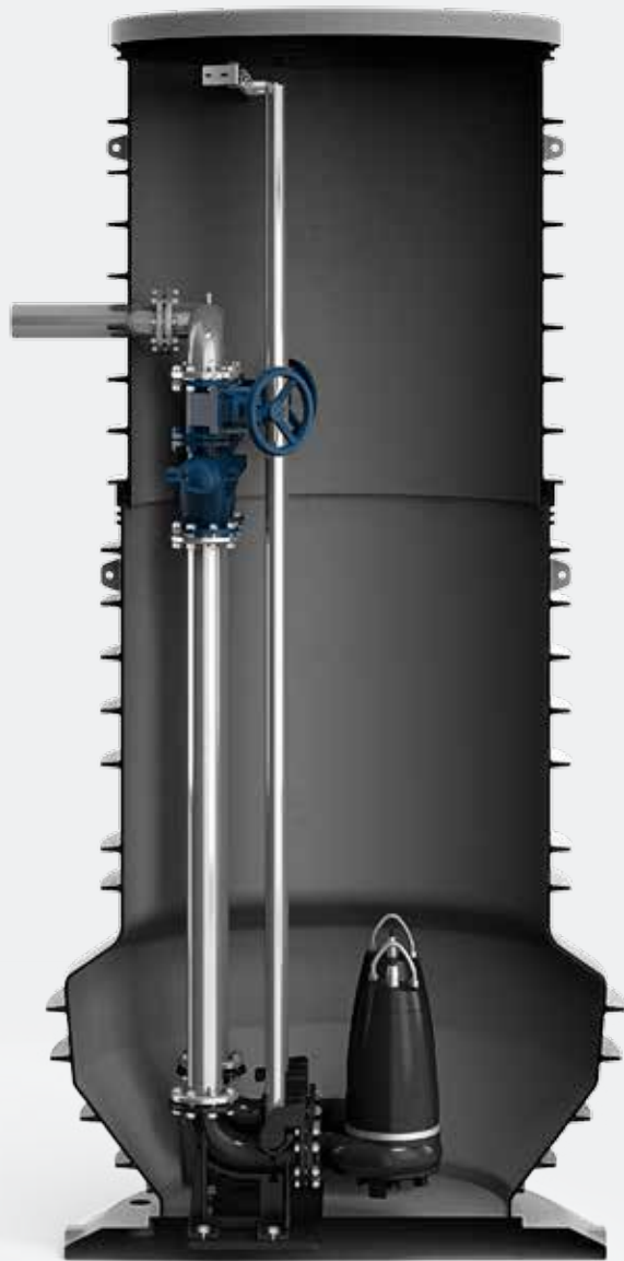
Fig. 7 Pumping stations for double installation of submersible sewage pumps on auto-coupling system. Sump diameter 1700 and main section diameter 1400 mm. Total length 2000 mm to 6000 mm
