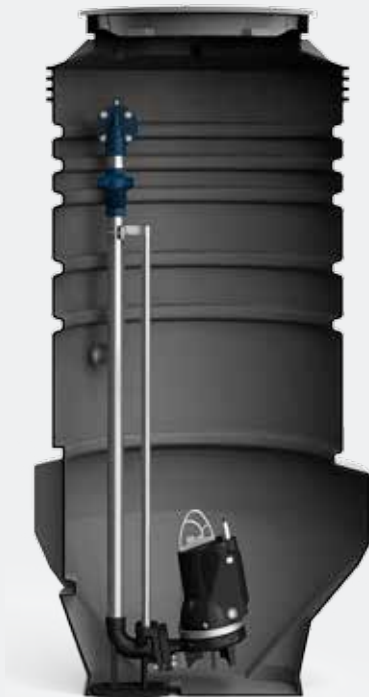
Fig. 4 Pumping station for single installation of a submersible SEG AUTOADAPT grinder pump on auto-coupling system. Sump diameter 800 and main section diameter 600 mm
