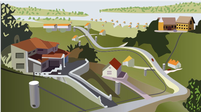
Fig. 2 Pressurised sewer system with grinder pumps in a remote area with undulating ground.
