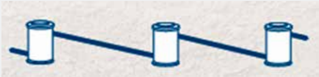
Fig. 8 Gravitation sewer system
