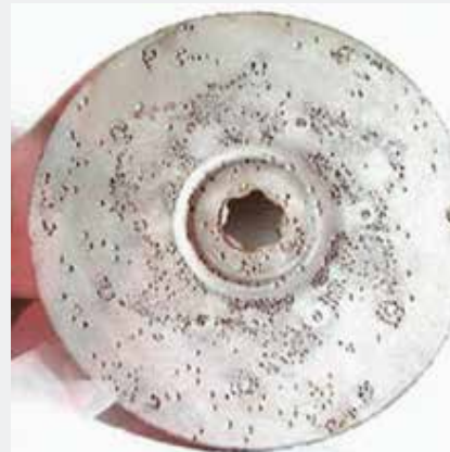
Fig. 5 Typical cavitation pitting on the backside of the impeller
