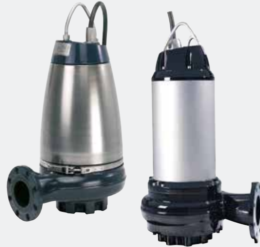
Fig. 2 Grundfos submersible SE pumps with motor jacket and cooling system can operate continuously with a liquid level down to the top of the pump housing
