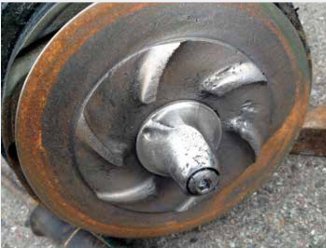
Fig. 11 Grinder pump with grinder system and impeller after one year of operation in an application with sand problems.
