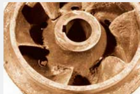
Fig. 6 Typical cavitation at the inlet to the impeller
