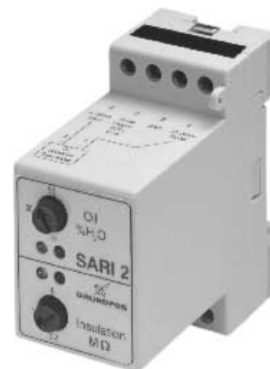
Grundfos SARI 2 monitoring device. The SARI 2 is mounted on a DIN rail in the control panel. The SARI 2 is intended for both stand-alone alarm use and for interfacing with a remote monitoring system.
